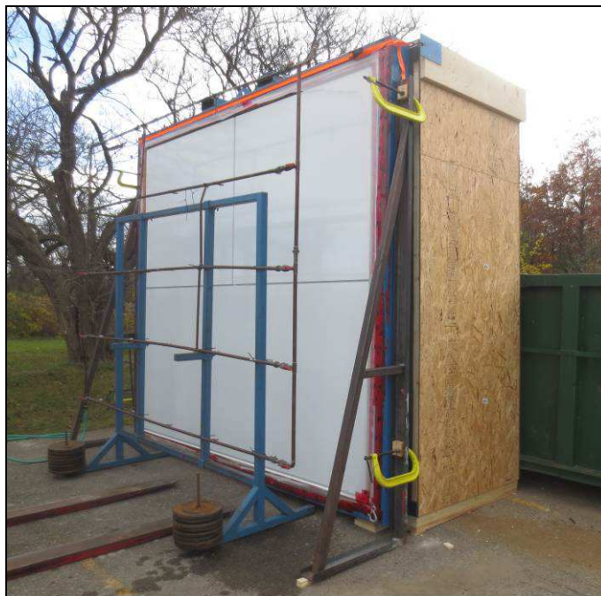
Figure C2 - Spray rack Set up for water penetration
